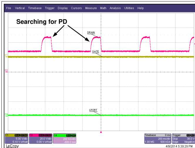
Figure 51. Open Circuit Detection
