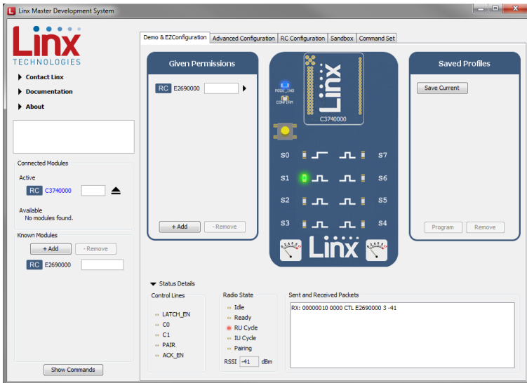
Figure 32: The Master Development System Software Receiving Module
