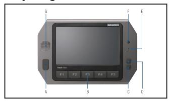
A. USB Host B. 5 programmable hotkeys C. D. Brightness control E. Power LED F. Light sensor G. Speaker
