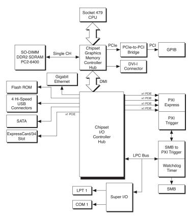
Figure 2. NI PXIe-8108 Block Diagram
