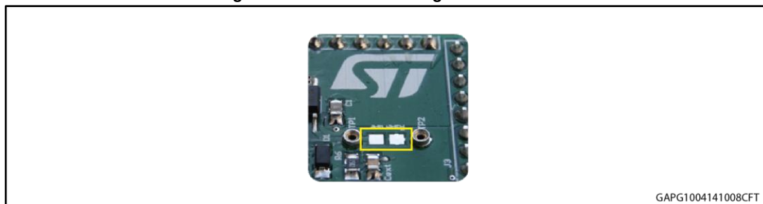
Figure 5: Pads for soldering SMD resistor
