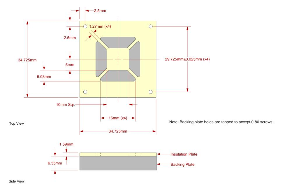
Description: <u>Backing Plate with Insulation Plate</u>
