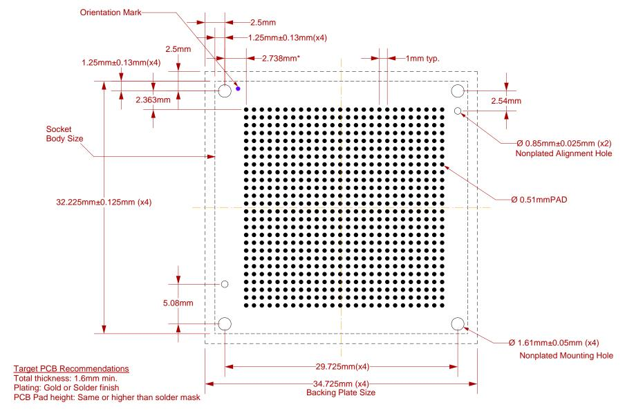
NOTE: Steel backing plate may be required based on end user's application
