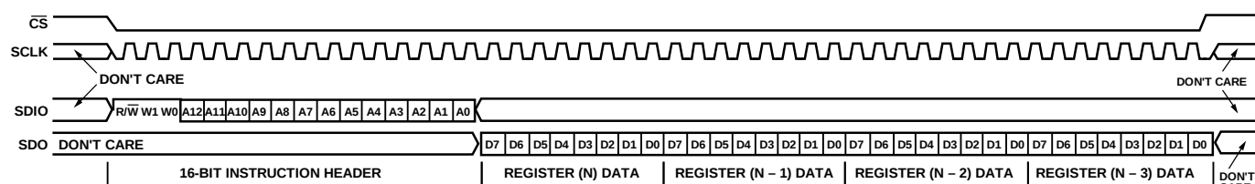
Figure 46. Serial Control Port Read—MSB First, 16-Bit Instruction, Four Bytes of Data
