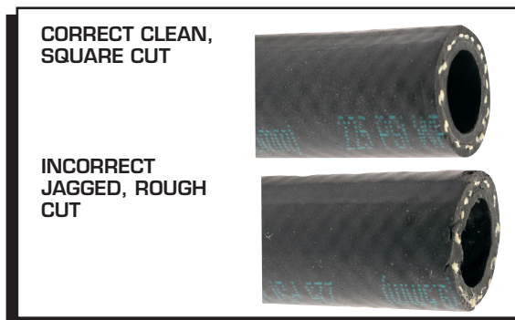
Figure 11 Severing the Hose Properly.
