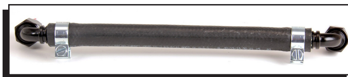
Figure 10 Installing Fuel Hose to AN Fittings.
