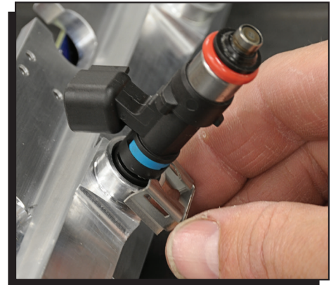
Figure 6 Installing the Injectors.
