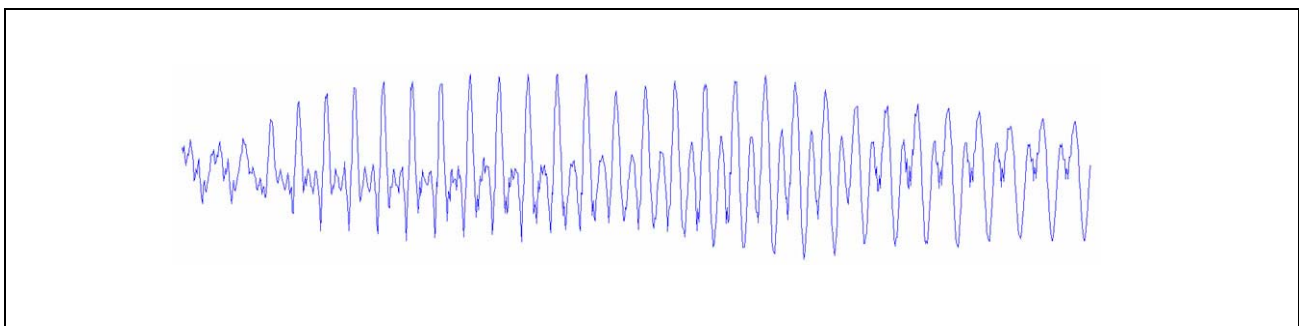
Figure 8: CVSD Decoder Output Waveform After Applying PLC
