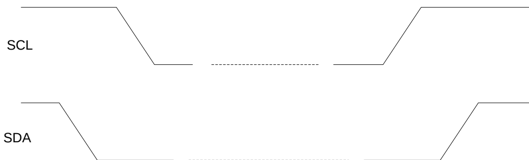
Figure 16: I 2 C START and STOP Condition Timing
