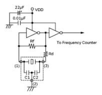
Regarding CERALOCK® with built-in capacitors, the terminal (1) and (3) are interchangeable, but if connection is interchanged, the specification of initial tolerance frequency may not be guaranteed. \*Please see dimensions about terminal numbers.
