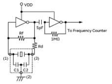
Regarding CERALOCK<sup>®</sup> with built-in capacitors, the terminal (1) and (3) are interchangeable, but if connection is interchanged, the specification of initial tolerance frequency may not be guaranteed. \*Please see dimensions about terminal numbers.
