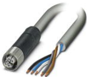
Power cable, 5-position, PVC, gray RAL 7001, Socket straight M12, L-coded, on free cable end, cable length: 5 m, for direct current up to 16 A/63 V
