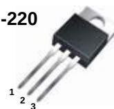
1.Gate 2. Drain 3. Source
