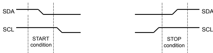
Figure 13-3. START and STOP Conditions
