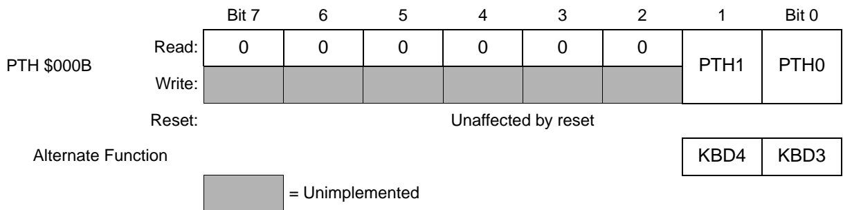
Figure 20-22. Port H Data Register (PTH)
