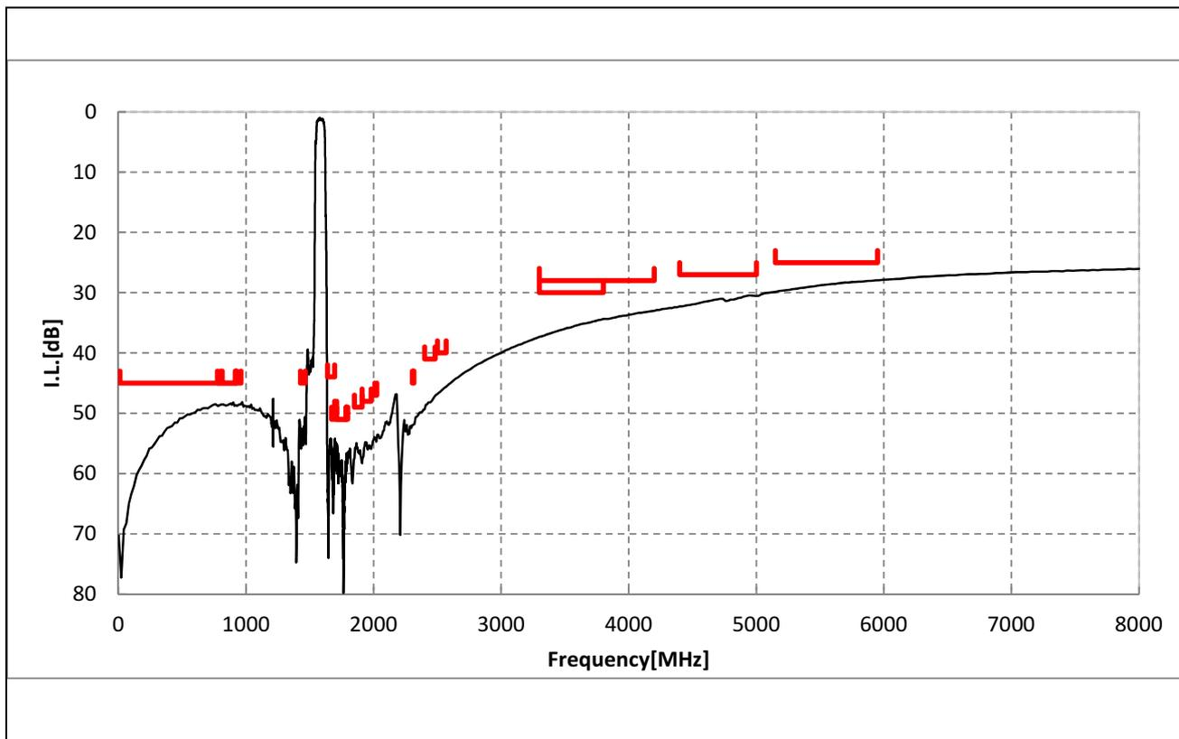
SAFFB1G56AC0F0A ( GPS\_GLONASS\_BEIDOU / Unbalanced / 5pin / 1109 )
