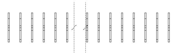
NOTE: CONTACTS ARE HELD IN A CARRIER FOR EASE OF ASSEMBLY
