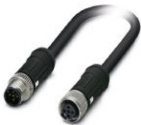
Sensor/actuator cable, 5-position, PE-X halogen-free, black, shielded, Plug straight M12 SPEEDCON, coding: A, on Socket straight M12 SPEEDCON, coding: A, cable length: 2 m, For railway applications
