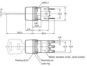
Dimensions • The Dimension shows 2-switch outputs. • The lamp terminal is also provided with non-lighted models. • A rectangular model is listed as an example. (Unit: mm)
