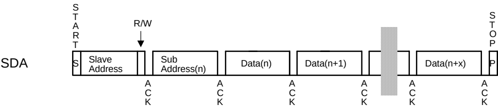
Figure 22. Data transfer sequence at the I 2 C-bus mode
