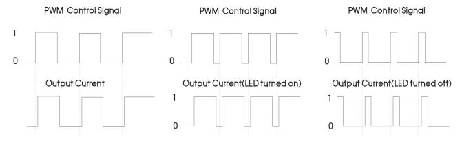
For PWM dimming signals with a certain frequency, the output current of the driver is related to the duty ratio of PWM signal. Refer to the formula for the calculation method:
