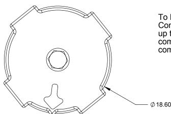
To be used with swivel lid sockets. Compression screw needs to be turned clockwise up to the point where the arrow on top of the compression screw aligns with laser mark on the compression screw bottom.
