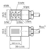
① Minimum bend radius at dynamic use  $R_{Min} = 20 x$  cable diameter
