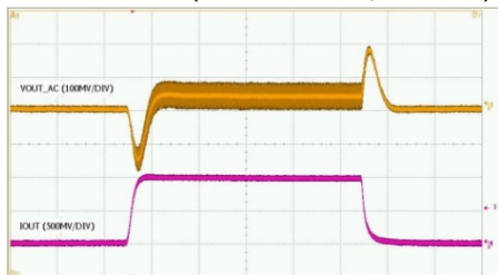
Load Transient (V IN =3V, PWM, I O =0A to 1A)
