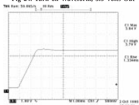
Fig 24. Turn on Waveform, 3.5 Volts Out
