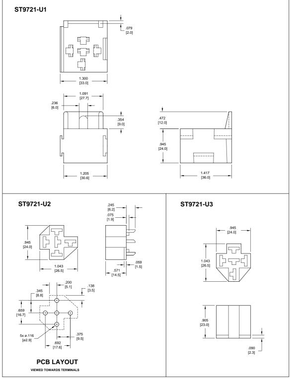
Note: Recommended receptical connector Amp Part numbers are 5-160558-9 or 5-1605-26-9
