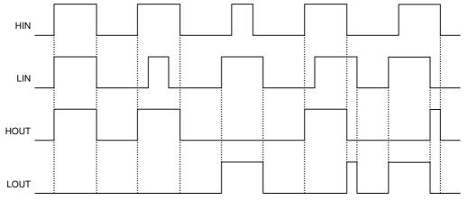
Note1: The minimum input pulse width at HIN/LIN should be to more than 500ns (because of HIN/LIN input noise filter circuit).
