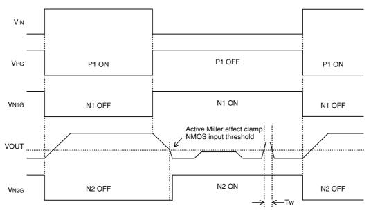
Active Miller effect clamp NMOS keeps turn-on if Tw does not exceed active Miller clamp NMOS filter time
