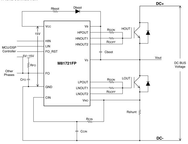
Note: If HVIC is working in high noise environment, it is recommended to connect a 1nF ceramic capacitor (CFO) to FO pin.
