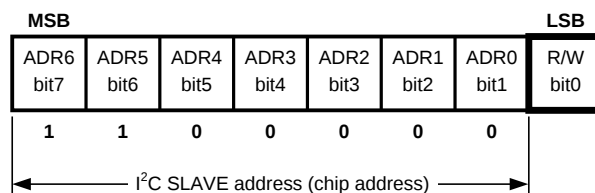
Figure 36. I 2 C Chip Address
