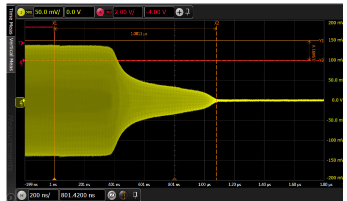
Figure 15. Switching Time [Insertion Loss to Isolation State]
