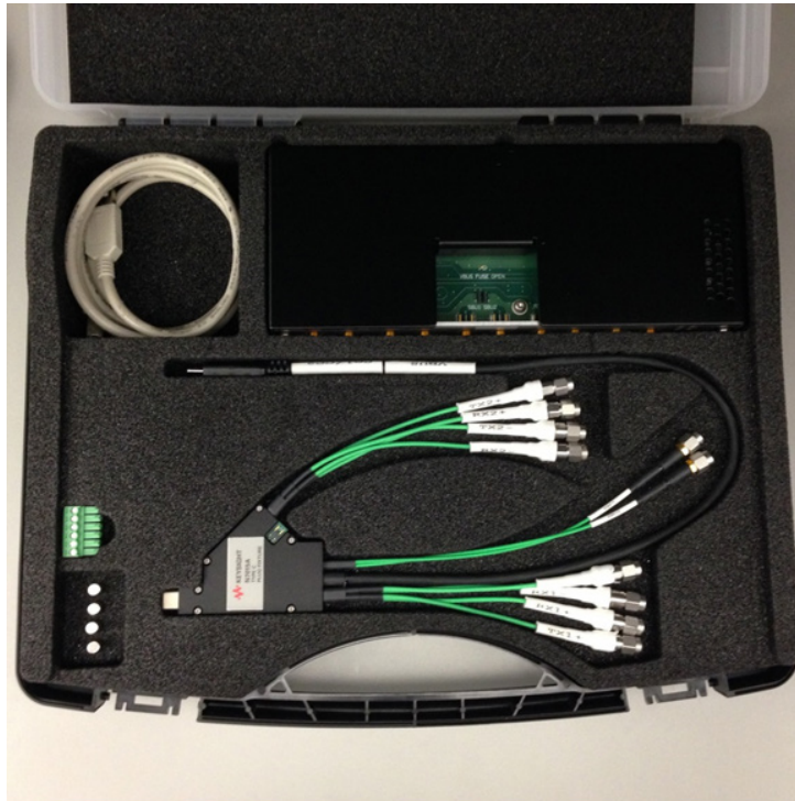
Figure 20. The Keysight N7015A USB Type-C Test Point Adapter Fixture.
