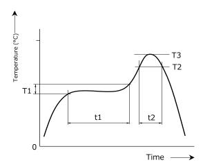
Pb free solder recommended temperature profile Voltage Step-up Coils
