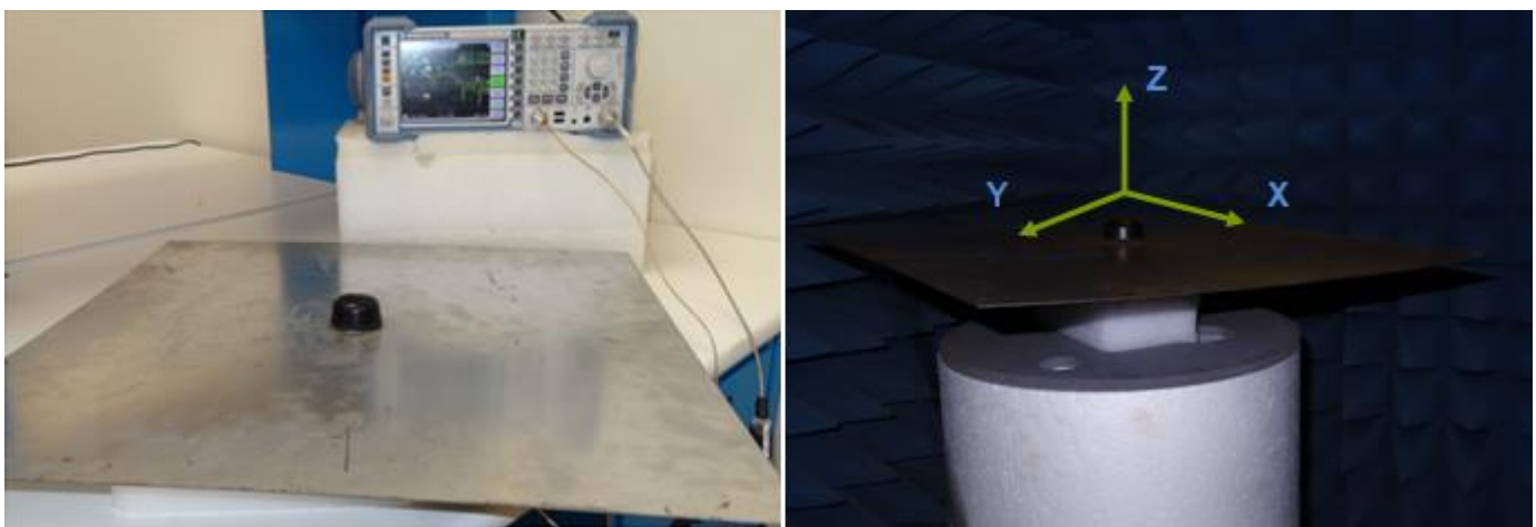
Figure 1. Impedance measurement (left hand) and efficiency, gain, radiation pattern measurements (right hand).
