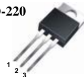
1.Gate 2. Drain 3. Source
