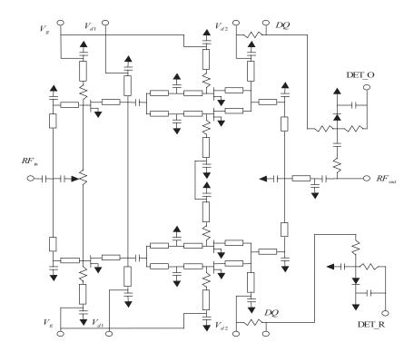
Figure 11. AMMC-6420 Schematic
