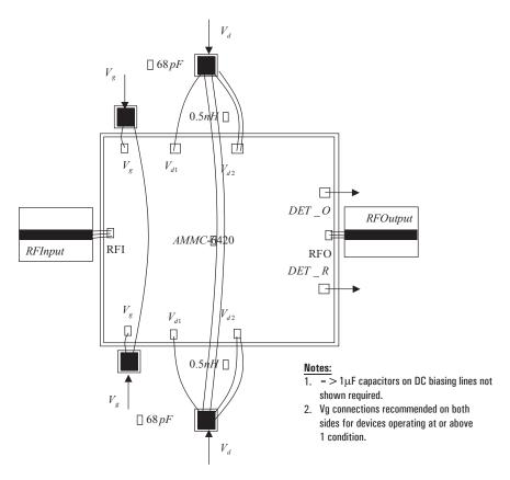
Figure 13. AMMC-6420 Assembly diagram
