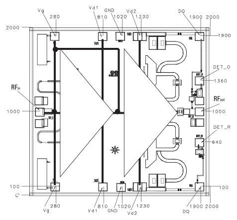
Figure 12. AMMC-6420 Bonding pad locations
