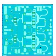
Chip Size:  $2000 \times 2000 \ \mu m$  (78.5 x 78.5 mils) Chip Size Tolerance:  $\pm$  10  $\mu m$  ( $\pm$ 0.4 mils) Chip Thickness:  $100 \pm 10 \ \mu m$  ( $4 \pm 0.4 \ mils$ ) Pad Dimensions:  $100 \times 100 \ \mu m$  ( $4 \pm 0.4 \ mils$ )
