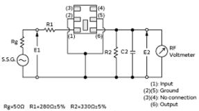
C2=10±2pF (Including stray capacitance and Input capacitance of RF voltmeter) E1: S.S.G. Output Voltage
