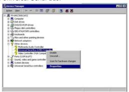
3. The PCI Universal Serial Bus Properties screen then appears, allowing you to re-install the driver. Select Driver from the main menu to proceed.
