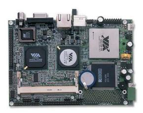
The HS-2606 is a 100/133MHz FSB VIA CLE266/VT8235 chipset-based board designed for Mini PCI Local Bus VIA Eden 1GHz Embedded CPU. These features combine and make the HS-2606 and ideal all-in-one industrial single board computer. Additional features include and enhanced I/O with CF, PCMCIA, CRT/Panel, audio, LAN TV-Out, 4 COM, and USB2.0 interfaces.
