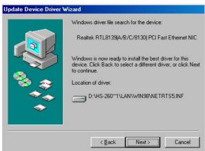
9. The program then copies the necessary files from your Windows installation disk to complete the driver setup process. Once the driver is completely installed, the following message appears on your display. Click on the Finish button to proceed.
