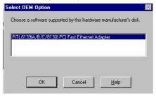
8. Setup then returns to Network Setup Wizard screen and displays your new Network Adapter. Click on Next to continue.
