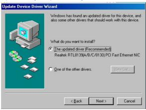
8. Once the program detects the device driver (\*.inf) file from your specified location, it will automatically copy the files into your hard drive.
