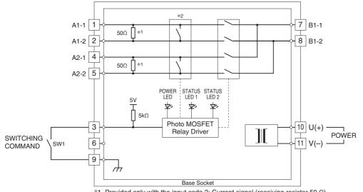
\*1. Provided only with the input code 2: Current signal (receiving resistor 50  $\Omega$ ). \*2. Provided only with the input code 1: Current signal (no receiving resistor).
