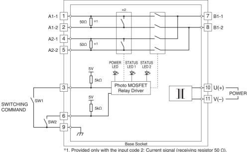
\*1. Provided only with the input code 2: Current signal (receiving resistor 50  $\Omega$ ). \*2. Provided only with the input code 1: Current signal (no receiving resistor).
