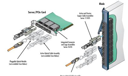
Passive Optical Cable Assembly Series 106284 (Series 106005 not shown above)
