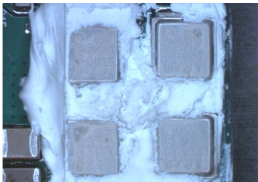
Figure 15 Excess heatsink adhesive covering devices
