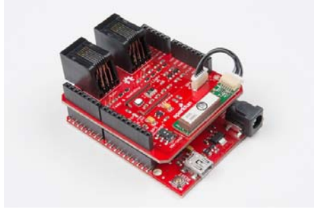
Shield on a RedBoard with optional weather meter connectors and GPS attached
