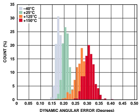
图8. 动态角度误差,  $V_{DD} = 2.7\text{ V}$ , GC = 关
