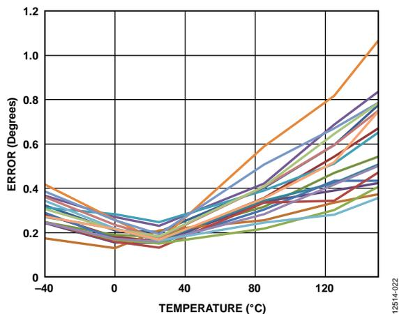
图15. 单点校准角度误差,  $V_{DD} = 2.7\text{ V}$ ,  $GC = \text{开}$
