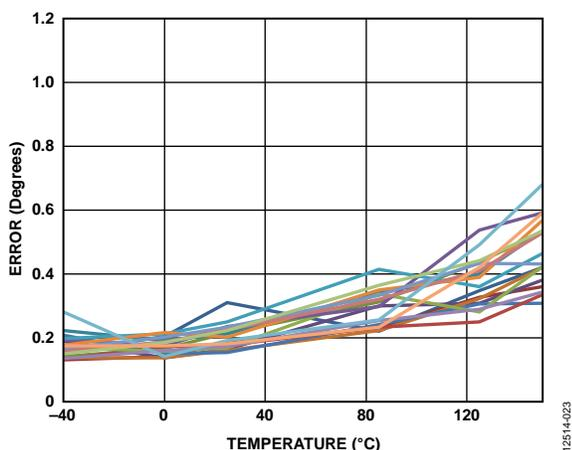
图16. 单点校准角度误差,  $V_{DD} = 2.7\text{ V}$ ,  $GC = \text{关}$
