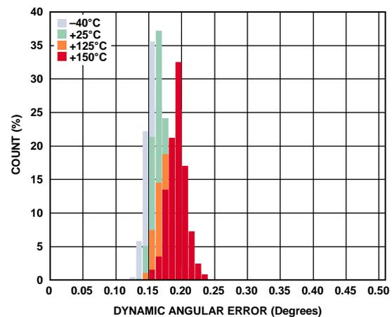
图5. 动态角度误差,  $V_{DD} = 5.5\text{ V}$ , GC = 开
