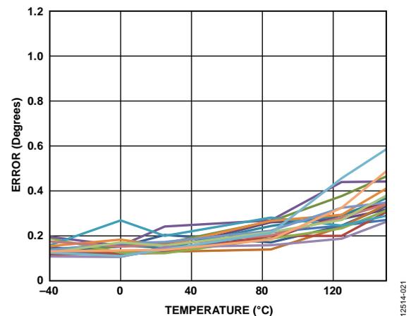
图14. 单点校准角度误差,  $V_{DD} = 5.5\text{ V}$ , GC = 关
