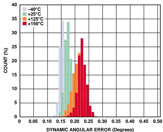
图6. 动态角度误差,  $V_{DD} = 5.5\text{ V}$ , GC = 关
