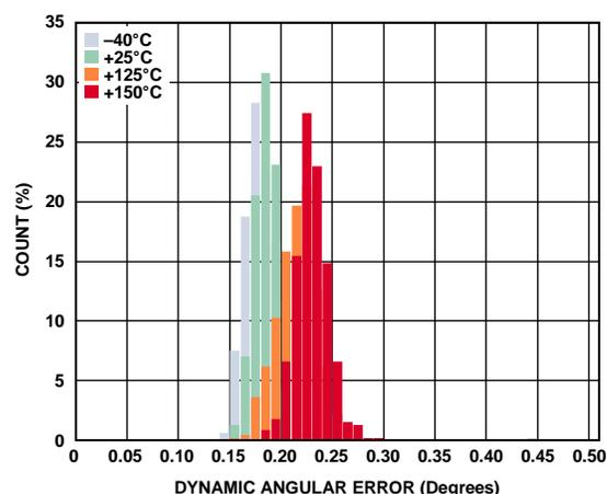
图7. 动态角度误差,  $V_{DD} = 2.7\text{ V}$ , GC = 开
