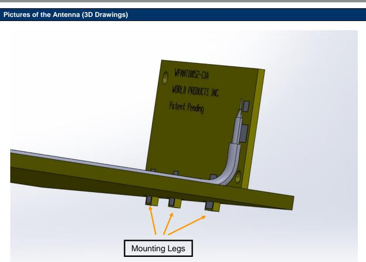
**Note**: There is no need for any additional Cables or Connectors. This eliminates the possibility of additional overhead for the Clients. Antenna is soldered directly in place on the Eval board.
