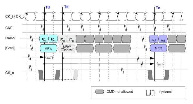
NOTE 1 Optional MRW RESET command and optional CS assertion are allowed, When optional MRW RESET command is used, tINIT4 starts at Td'.
