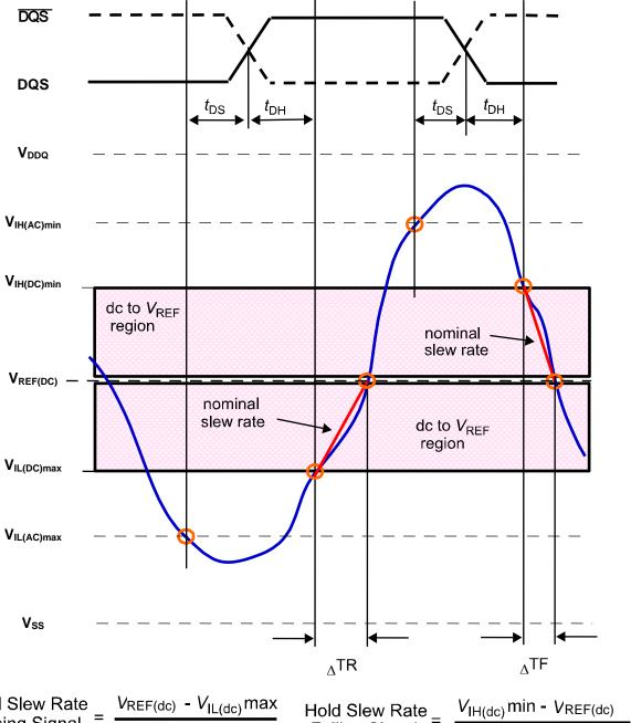
$$\frac{\text{Hold Slew Rate}}{\text{Rising Signal}} = \frac{V_{\text{REF(dc)}} - V_{\text{IL(dc)}} \text{max}}{\Delta^{\text{TR}}} \qquad \frac{\text{Hold Slew Rate}}{\text{Falling Signal}} = \frac{V_{\text{IH(dc)}} \text{min} - V_{\text{REF(dc)}}}{\Delta^{\text{TF}}}$$
