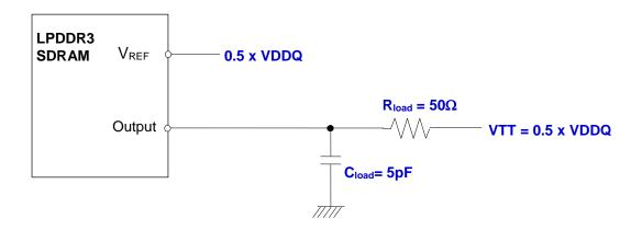
NOTE 1 All output timing parameter values (tDQSCK, tDQSQ, tHZ, tRPRE, etc.) are reported with respect to this reference load. This reference load is also used to report slew rate.
