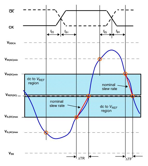
$$\frac{\text{Hold Slew Rate}}{\text{Rising Signal}} = \frac{V_{\text{REF(dc)}} - V_{\text{IL(dc)}} \text{max}}{\Delta \text{TR}} \qquad \frac{\text{Hold Slew Rate}}{\text{Falling Signal}} = \frac{V_{\text{IH(dc)}} \text{min} - V_{\text{REF(dc)}}}{\Delta \text{TF}}$$
