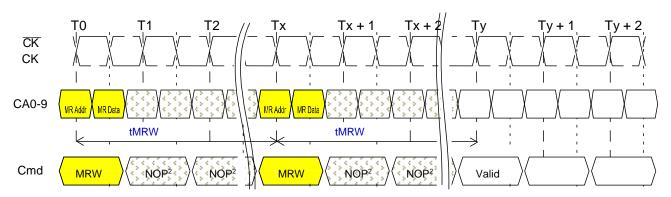
NOTE 1 At time Ty, the device is in the idle state.
