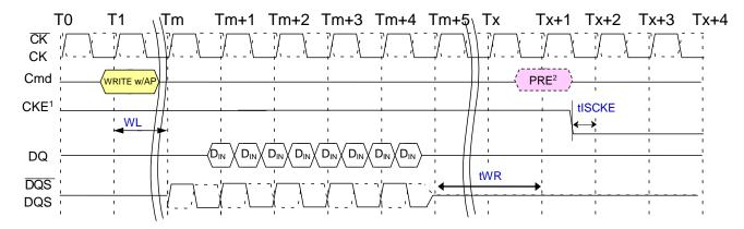
NOTE 1 CKE can be registered LOW at WL + 1 + BL/2 + RU(tWR/tCK) + 1 clock cycles after the WRITE command is registered.
