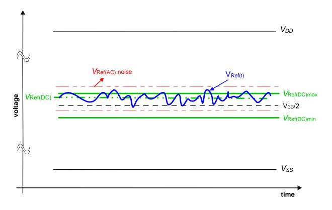
The voltage levels for setup and hold time measurements  $V_{IH(AC)}$ ,  $V_{IH(DC)}$ ,  $V_{IL(AC)}$  and  $V_{IL(DC)}$  are dependent on  $V_{Ref}$ . " $V_{Ref}$  "shall be understood as  $V_{REF(DC)}$  above.
