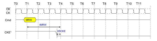
${\tt NOTE~1} \quad {\tt CKE~can~be~registered~LOW~tMRW~after~the~clock~on~which~the~MRW~command~is~registered}.$
