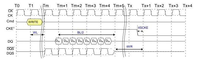
NOTE 1 CKE can be registered LOW at WL + 1 + BL/2 + RU(tWR/tCK) clock cycles after the clock on which the WRITE command is registered.
