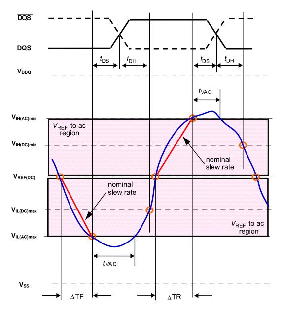
Setup Slew Rate Falling Signal =
