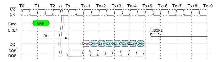
NOTE 1 CKE can be registered LOW RL + RU(tDQSCK/tCK)+ BL/2 + 1 clock cycles after the clock on which the MRR command is registered.
