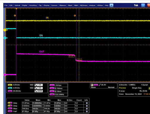
Figure 9-5. OUT In Current Fault Auto Recovery, High Side Mode
