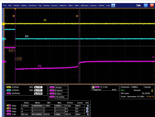
Figure 9-4. OUT In Current Fault Auto Recovery, Low Side Mode
