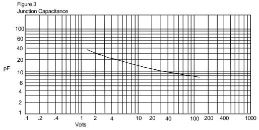
Junction Capacitance - pF versus Reverse Junction Potential (Applied V + 0.7 Volts) - Volts
