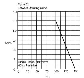
Average Forward Rectified Current - Amperes versus
