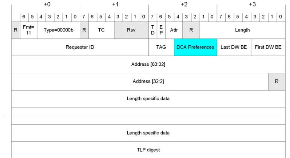
Figure 3-41. PCIe Message Format for DCA
