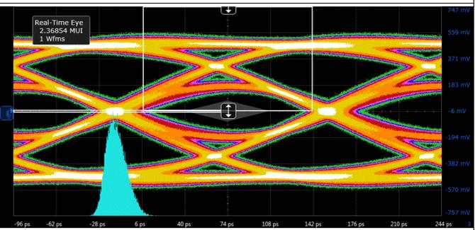
Figure 18. HDMI2.0 6-Gbps TP2 Eye Diagram (With TPD4E02B04)
