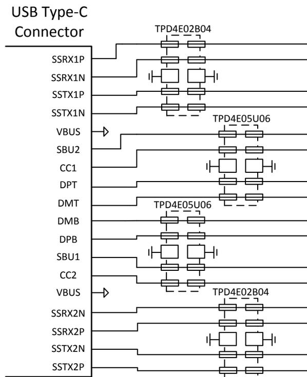
**Figure 20. USB 3.1 Gen 2 Type-C ESD Schematic**
