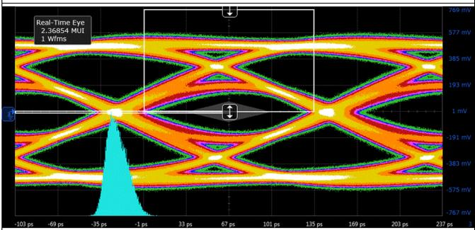
Figure 17. HDMI2.0 6-Gbps TP2 Eye Diagram (Bare Board)
