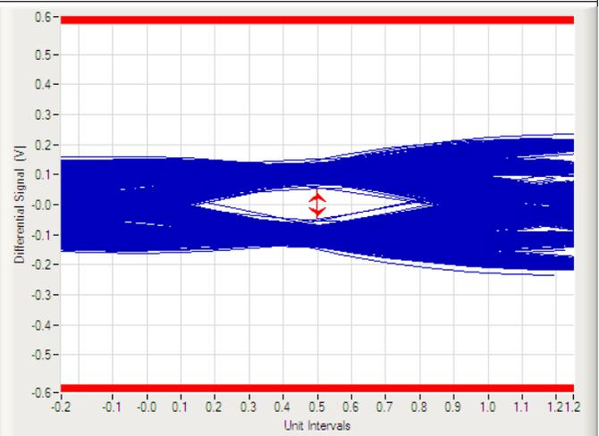
Figure 16. USB3.1 Gen 2 Eye Diagram (With TPD4E02B04)
