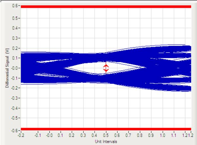
Figure 15. USB3.1 Gen 2 Eye Diagram (Bare Board)
