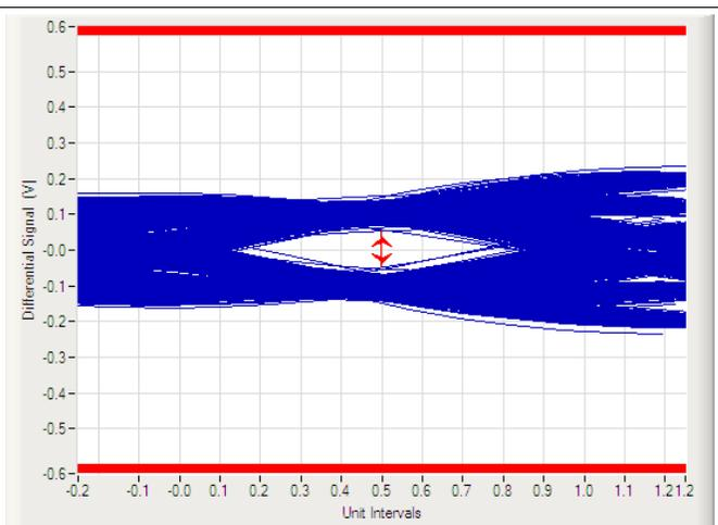
**Figure 23. USB 3.1 Gen 2 10-Gbps Eye Diagram (With TPD4E02B04)**
