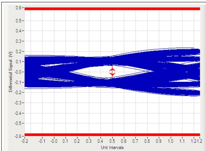
**Figure 22. USB 3.1 Gen 2 10-Gbps Eye Diagram (Bare Board)**
