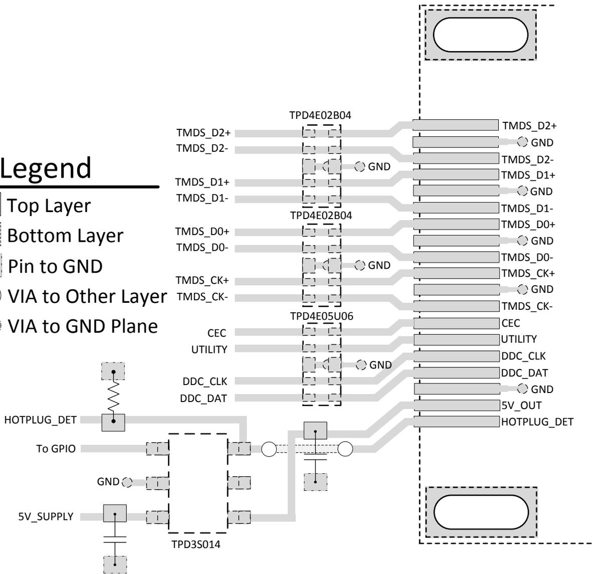
Figure 25. HDMI2.0 Type-A Transmitter Port Layout
