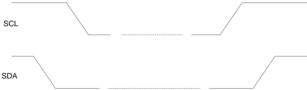
Figure 16: I 2 C START and STOP Condition Timing
