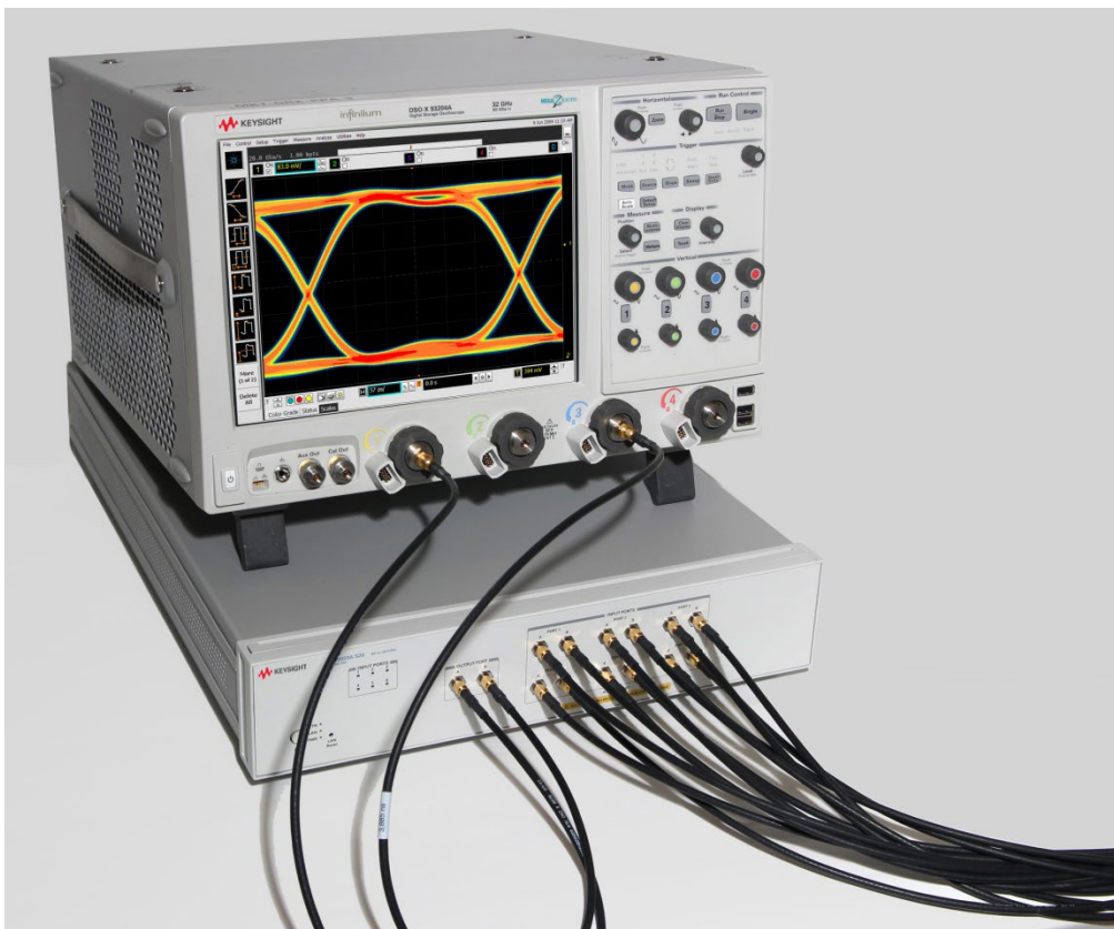
Figure 9. Automated testing for multi-lane digital bus interface through switching solution.
